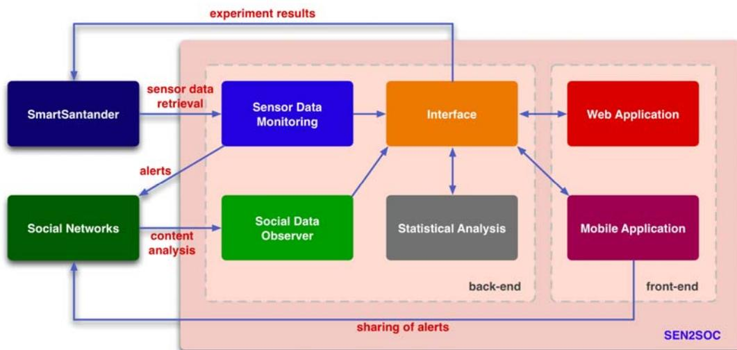
Figure 1 : The SEN2SOC architecture
